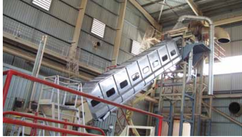
Lint Slide that Orange Precision built for Queensland cotton in Wee Waa
